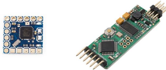
Figure 14. Example OSD Modules
