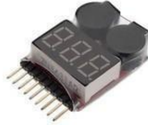
Figure 14: Sample Battery Alarm
