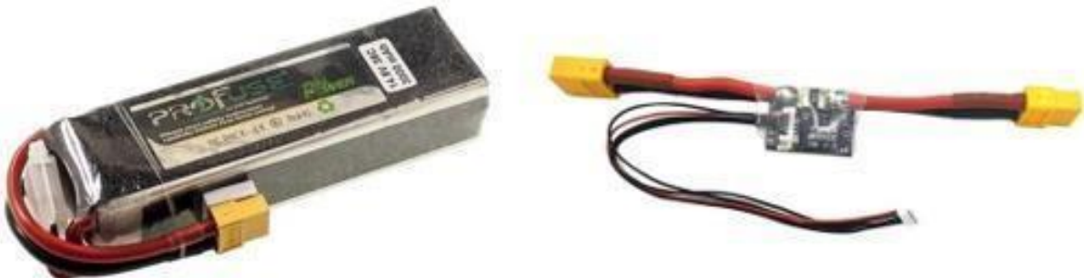
Figure 9: LiPo battery and power distribution module
